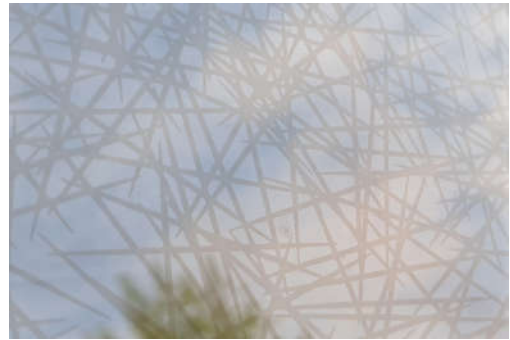
Figure 2: Bird friendly glass with UV light reflecting structures
